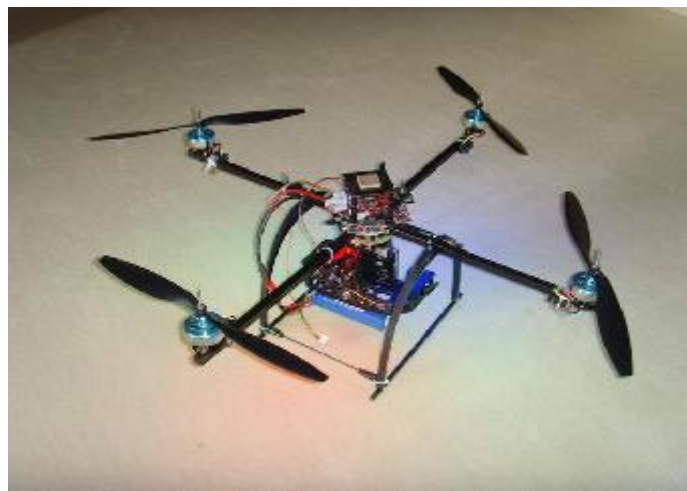
Figure 1. Mikrocopter configured in a four propellor set. Font: http://gallery.mikrokoetter.de/main.php/v/Nachbau/z.JPG.html
